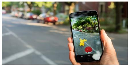
Content is drawn on top of a camera's video input. A person sees their "normal" environment though the camera, with additional graphics in it.
